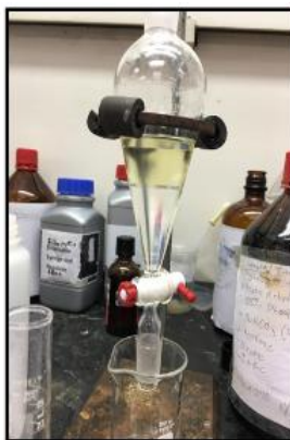
Figure 5: Separation of organic layer by workup procedure
